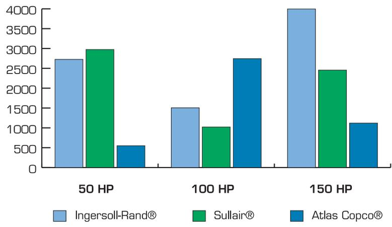
Calculations (using published data) are based on the cost of providing the volume of air that Gardner Denver Electra-Saver II compressors can deliver in 8000 hours (approximately 1 year) of operation at full load. Assumes motor efficiency=.90, cost per kilowatt-hour=\$0.07.
